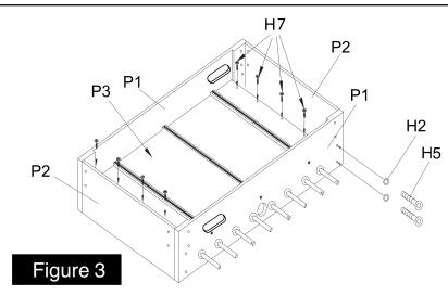
Attach the two end panels P2 as shown in FIGURE 3 using bolts H5 and washers H2. Remember to start all bolts by hand first before you tighten anything.
