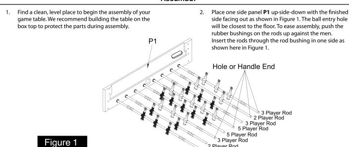
3. Align the rods as shown in **FIGURE 1**. Choose one team to be color # 1 and one team to be color # 2. The handle end of the rod has a hole close to the end of the rod. There will be four handles (one team) on each side of the table. Remember, the goalie rod is always in your left hand when the table is in the upright position and you are working upside down so it will be opposite during assembly.
