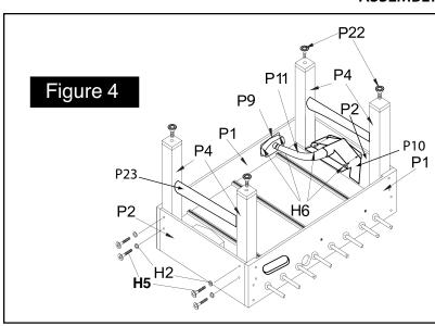
Attach legs as shown in FIGURE 4 using bolts H5 and washers H2. Attach Support Beam P23 to legs before tightening leg bolts. Remember to start all bolts by hand before you tighten the legs.
