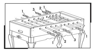
handle to the left, (#1) handle to the right, (#2) handle to the left, (#1) handle to the left. Do NOT attach rod end caps.
